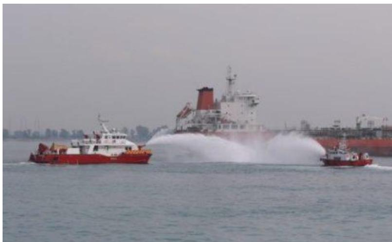
*Photo: water curtain dispersing the simulated Xylene fumes*
